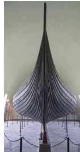
Left: A Viking longship showing the overlapping clinker planking.
